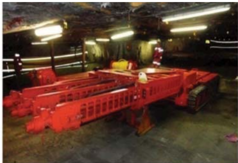
Figure 10 – ULP drill rig
