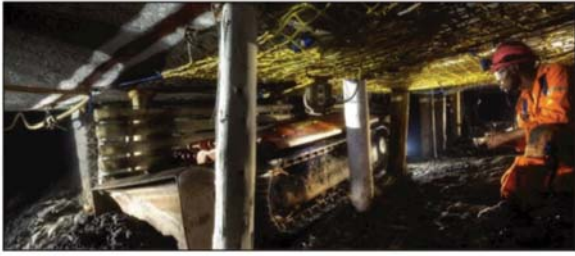
Figure 8 – ULP dozer cleaning a panel
