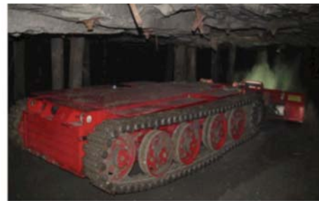
Figure 11 – ULP sweeper cleaning a panel
